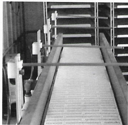
Flats are placed on the belt and seed are watered using this machine.
