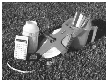
This is all you need to calibrate a sprayer. Photo credit: Erdal Ozkan
