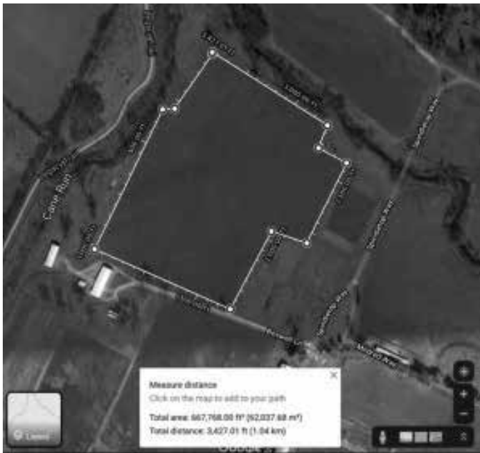
Figure 1. Mapping program, like Google Maps, can be used to determine the area of irregular-shaped fields.
