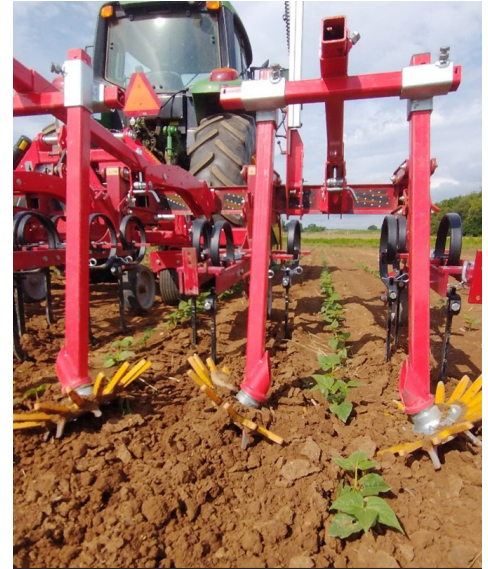
Figure 1. Cultivator setup using camera guidance to direct finger-weeder cultivators at V1-2 crop growth stage.
