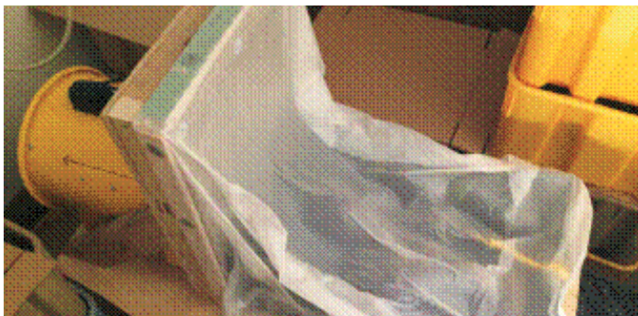
A countertop forced air cooler for 1-3 cartons of product. Photo credit: UVM Extension
