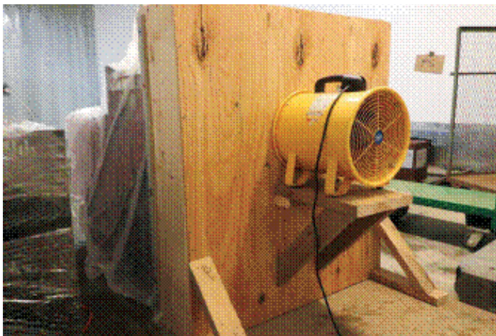
A countertop forced air cooler for 1-3 cartons of product. Photo credit: UVM Extension
