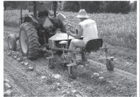
Eco Weeder for close cultivation around individual plants
